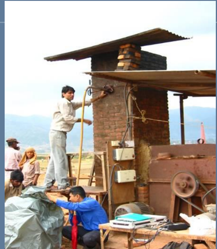
9 tones Coal & 180 KWH Electricity Consumption: / 100'000 bricks
